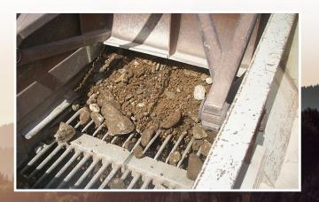
GRIZZLY SPRING FINGERS ARE DESIGNED SPECIFICALLY FOR EACH MACHINE AND BUILT TO INSTALL EASILY IN ALL MAKES OF VIBRATORY GRIZZLY FEEDERS AND SREENING APPLICATIONS.
